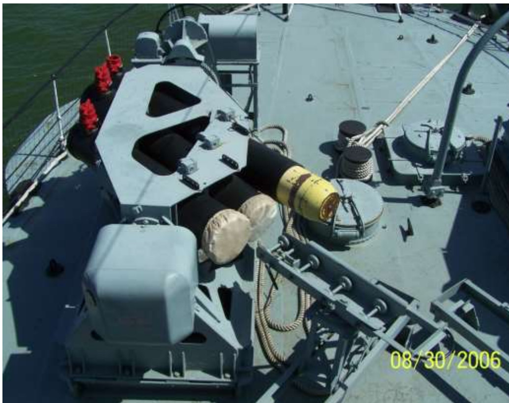
Squid on aft deck of HMCS HAIDA showing yellow Mortar and loading carriage.
